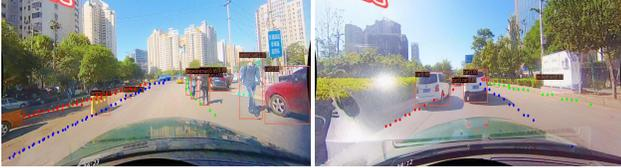
Figure 8: Performance in shadow and no-line conditions after image enhancement.
