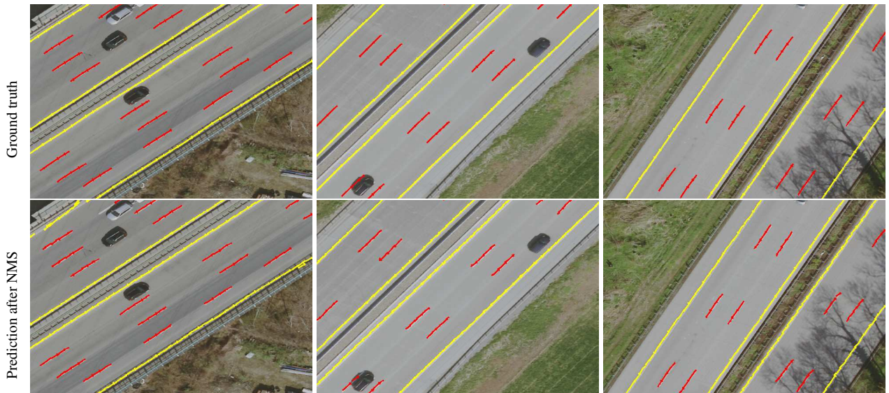
Figure 6. Results for the KAI dataset. The network has eight predictors, 16 px cells and unbound Cartesian points. Colors indicate the different classes: dashed and solid road marking. Aerial images: © City of Karlsruhe | Liegenschaftsamt
